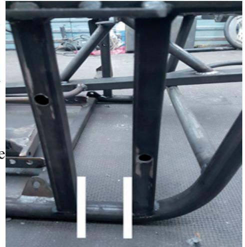
•To increase protection to the driver's footwell it is required as a minimum to add a horizontal bar made of 20mm x 20mm (2mm wall thickness) to each side of the footwell to make an 'H'. It is required to fit an extra vertical upright on one side to achieve this, which has a minimum specification of 25mm x 25mm (2mm wall thickness).
