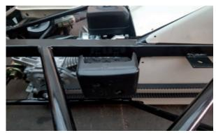
Once you run the Lifan LF210E engine, the exhaust MUST be on the outside of the car.
